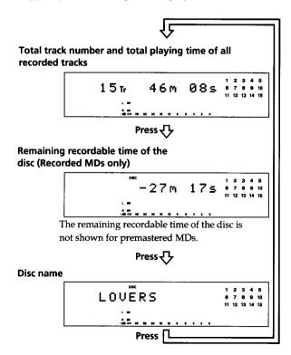
When you insert an MD, the disc name, total number of tracks, and total disc playing time appear in the display as follows:
