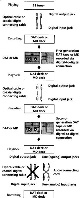
3 You can record a DAT tape or MD recorded via the DAT or MD deck's analog input jack onto another DAT tape or MD via the DAT or MD deck's digital output jack. You cannot, however, make a second-generation DAT tape or MD copy via the DAT or MD deck's digital output jack.
