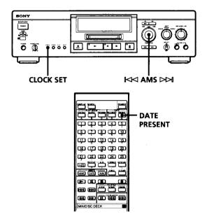
1 Press CLOCK SET down for about 2 seconds until the year indication in the display starts flashing.
