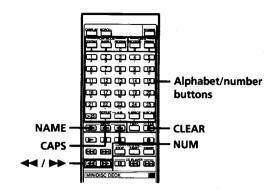
1 Press NAME repeatedly until a flashing cursor appears in the display, then do the following:
